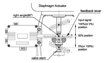
③ The stroke range for the best performance should be 5⊠ 80mm (optional 70~150mm) and the operation angle of the feedback lever should be less than Max. 45° to carry out accuracy and linearity perfectly.
