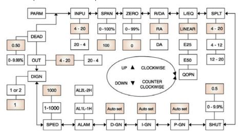
A Colored sub-parameters under main parameters are the factory settings. They will be restored to the defaults (factory settings) after RESET.
