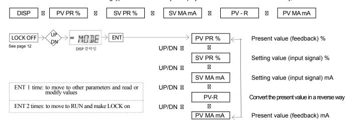
⚠ If PV-R is selected, one point is displayed on LCD. (See the circle of the below picture)
